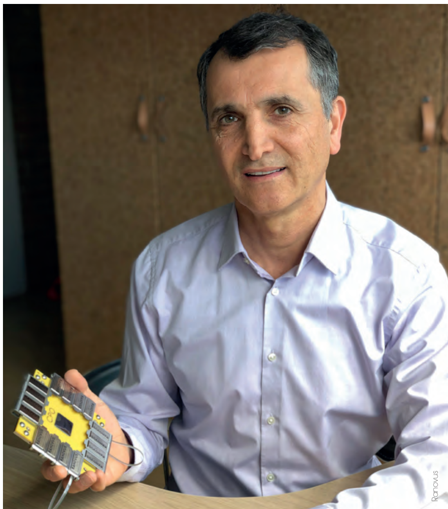
■ Ranovus' Odin IC has demonstrated operation with eight optical channels of 100Gbps per fibre pair, potentially enabling 25.6TbE switches
