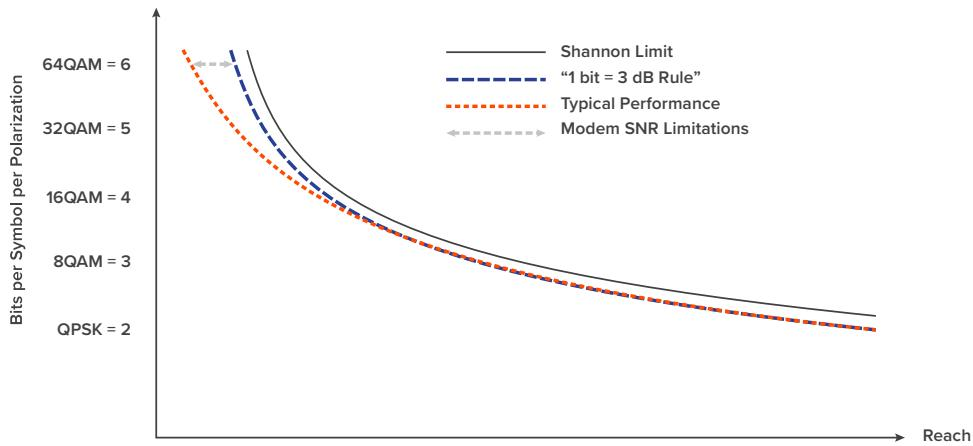
*Figure 4: Modulation (bits per symbol per polarization) vs. reach*
