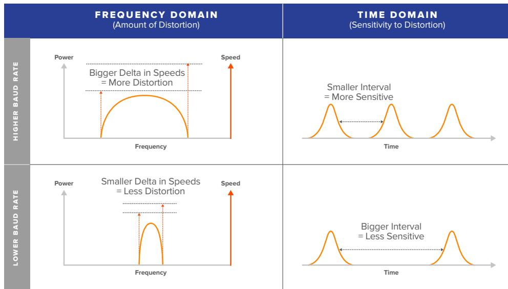
Figure 8: Baud rate and chromatic dispersion
