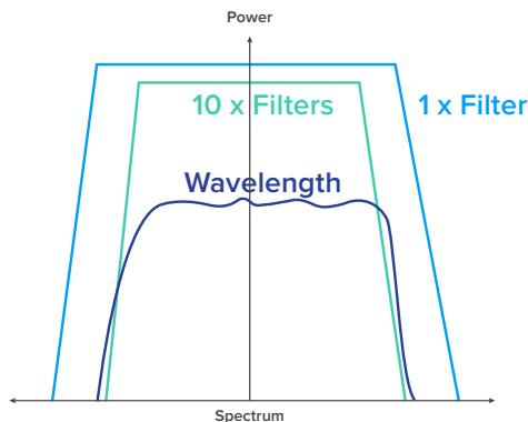
Figure 2: Filter penalties and filter narrowing
