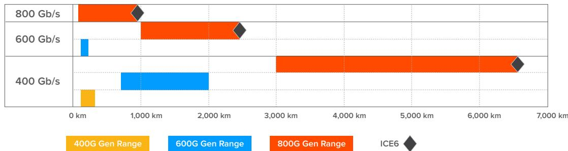
*Figure 16: ICE6 capacity-reach comparison*
