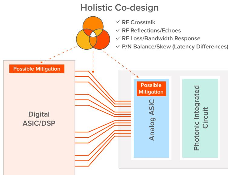
Figure 15: Holistic co-design of the critical RF interconnect
