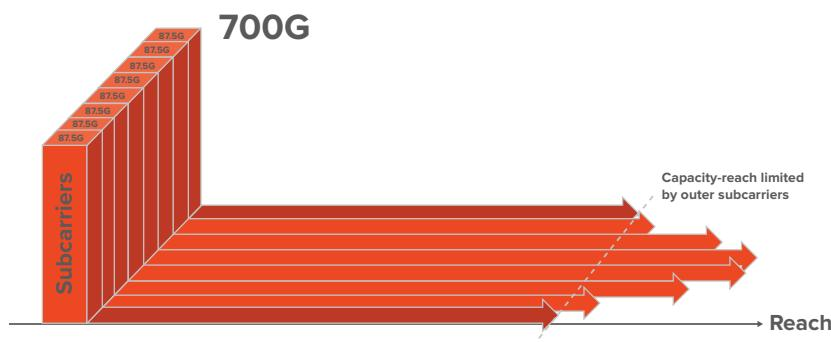
Figure 11: Without DBA, capacity-reach is limited by outer subcarriers
