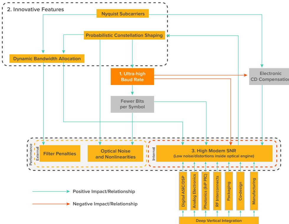
Figure 3: Key enablers of ICE6 wavelength capacity-reach
