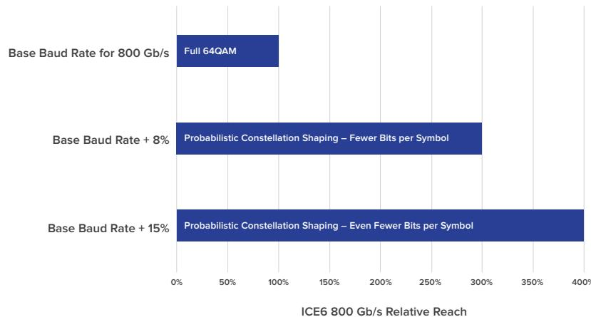
*Figure 5: 800 Gb/s wavelengths: ICE6 reach vs. baud rate*
